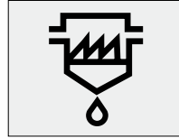
Oil-water separator warning lamp
