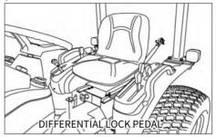
The differential lock is a device to lock the differential system in order to rotate the left and right wheels at the same speed.
