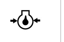
If the oil pressure lamp comes on check the oil level first of all.
