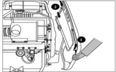
To open the side cover, grab it and pull the forward panel upward to separate from guide the support pin (1). And pull the side panel forward again.
