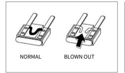
The circuit has blade type fuses in its wiring circuit.
