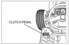
When the clutch pedal is pressed on models with mechanical transmissions, drive is disengaged and the gear range and forward or reverse travel can be selected.
