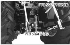
If the PTO is not used, grease it and install the PTO shaft cap.
