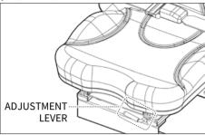
Before operating a tractor it is important to adjust the seat to the most comfortable position & check whether it is properly locked in its position.
