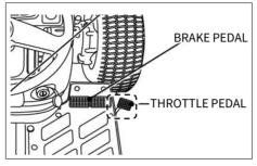
This pedal can override a fixed hand throttle setting.
