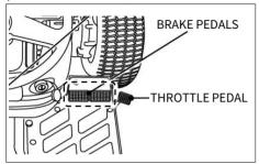
The brake pedals are used to stop the vehicle forcibly or turn the direction.
