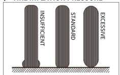
Check if the inflation pressure of the front and rear tires is correct. If not, adjust it to the specification.
