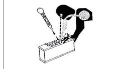
Sulfuric acid in battery electrolyte is poisonous.
