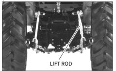
Adjust the length of the lift rod by screwing the adjusting handle (turnbuckle) in or adjust the length of the lift rod as necessary to set the implement in its working position parallel to the ground.
