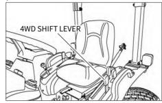
4WD lever is located below the LHS of the operator.
