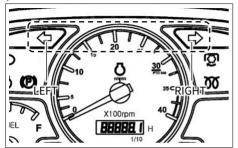
This lamp is used to indicate the intended turning direction of the driver. When pulling down the turn signal switch, the left turn signal lamp blinks. When pushing up the turn signal switch, the right turn signal lamp blinks. These lamps are operated when pressing the hazard warning lamp switch as well.
