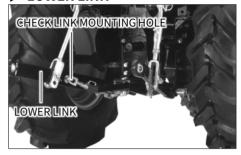
For different applications change the position of the yoke rod on the lower link holes as shown and insert the pin in the direction of the arrow.
