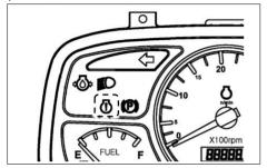
This comes on when engine is malfunctioning.
