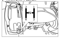
The main shift lever is located on the RHS of the operator.
