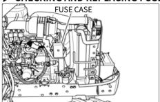
The wiring harness is equipped with main fuses whose function is to preserve the wiring.
