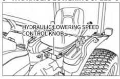
This can be used to adjust the lowering speed of the implement.
