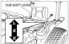
The sub shift lever provides two speed ranges of L and H.
