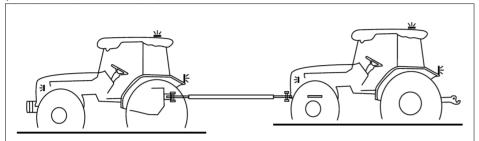
The tractor can be towed only for short distances, such as, for example, from inside to outside a building.
