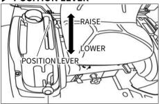
This lever is used to lift and lower an implement to a certain working height freely and maintain it.
