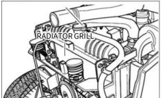
When working in a grassy field or working at night, the radiator or condenser grille may be clogged by grass, straws or bugs, reducing cooling performance.
