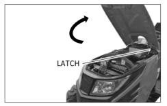
Lift the hood with hands. Then, the hood is automatically opened and fixed by its damper.
