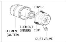
Check that the dust valve is not blocked. Inspect the rubber flaps for cuts and nicks and check that the rubber is not perished.
