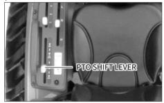
Only PTO lever is used to control PTO shaft.
