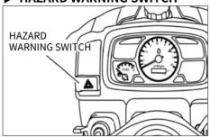
This switch can be used to warn other vehicles when malfunction occurs in the tractor while driving on public road. When pressing the switch once, left and right signal lights blink.
