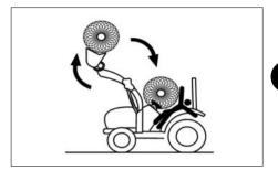
Never carry a big object with the loader unless a proper implement is attached.
