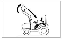
When attaching or detaching the loader, fix all parts which are connected to the bucket and boom.
