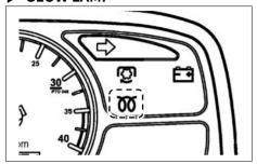
This comes on while the engine preheating function is activated. It goes off as soon as preheating is completed.
