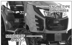
The engine and chassis number are stamped as shown in the drawing above.
