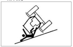
Do not drive where the tractor could slip or tip.
