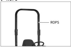
TYM tractors are equipped with a frame for the protection of operators. In the case of cab tractors the frame is incorporated in the cab structure. The objective of the frame or cab structure is to protect the operator in the event of a roll over and they are designed to support the entire weight of the tractor in that event.
