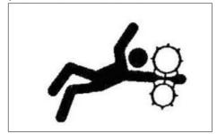
Do not wear a necktie, scarf or loose clothing when you work near moving parts.
