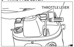
The throttle lever is used to change engine speed.
