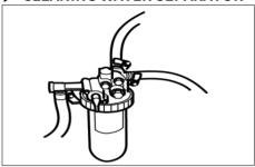
If any foreign material or water is seen through the sight glass, remove it by performing the following steps.
