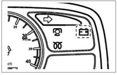
This lamp will go off as soon as the engine starts to run to indicate that the alternator is charging (Please note, as broken fan belt can cause the light to come on, please stop the engine as overheating can occur if not rectified immediately).
