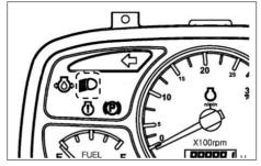
This lamp is operated on the combination switch.
