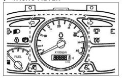
It displays the revolution of the engine or PTO shaft per minute.
