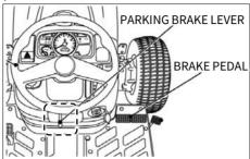
Push the brake pedals down while pulling the parking brake lever up to engage. Press the brake pedals to release parking brake.
