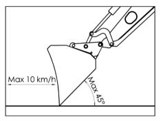
When leveling do not drive faster than 10 km/h. In this process tilt the implement a maximum of 45°.
