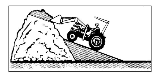
Another method for large dirt piles is to build a ramp approach to the pile.
