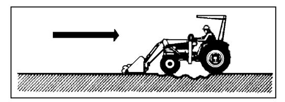
Backgrade occasionally with a loaded bucket to keep the working surface free of ruts and holes. Hold the lift control forward in FLOAT POSITION so the full weight of the bucket is scraping the ground. Use only the heel of the bucket while backgrading.
