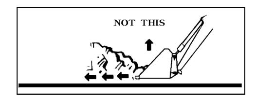
Note: Do not be concerned if the bucket is not completely filled during each pass Maximum productivity is determined by the amount of material loaded in a given period of time. Time is lost if two or more attempts are made to fill the bucket on each pass
