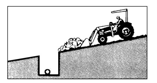
Pile dirt on the high side for easier backfilling on a slope
