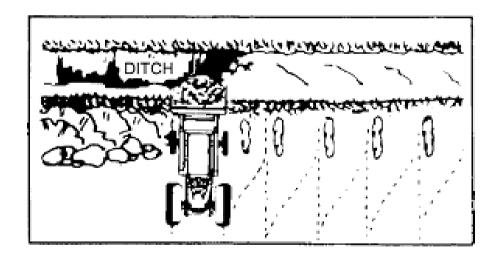
Leave dirt which drifts over the side of the bucket for final clean-up
