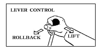
The lift and rollback of the bucket will increase efficiency because a level bucket throughout the lifting cycle resists bucket lift and increases breakaway effort.
