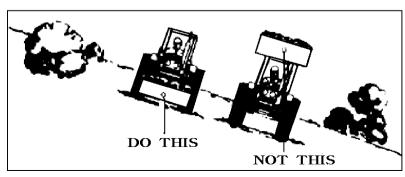
When transporting the load, Keep the bucket as low as possible to avoid tipping, in case a wheel drops in a rut.
