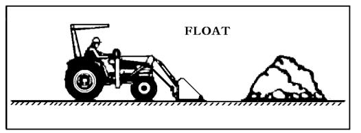
The float will also prevent the mixing of surface material with stockpile material. The float position will reduce the chance of surface gouging when removing snow or other material.
