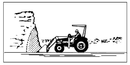
Exercise caution when under cutting high Banks.Dirt slides can be dangerous.Load from as low as possible for maximum efficiency.Loader lift and breakaway capacity diminish as loading height is increased
