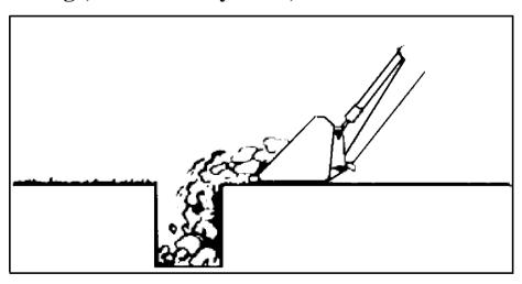
Leave dirt in the bucket because dumping on each pass wastes time.
