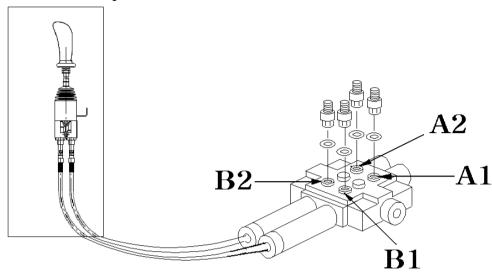
The single lever and joystick control lever is mounts on the tractor from the factory. The control lever has the safety lock function.
