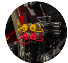
6. Rear external hydraulic valve
