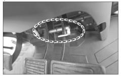
There is an interlock for connecting the left and right brake pedals.
