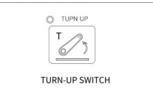
This function is to lift the implement automatically when the vehicle is being turned.
