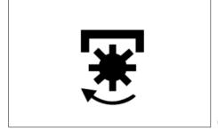
PTO lamp indicates the state of the PTO shaft.
