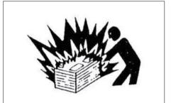
Keep sparks, lighted matches and open flame away from the top of battery. Battery gas can explode.
