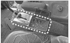
The electronically controlled lift system can provide various functions through simple switch operations, unlike the mechanical type, to enhance the driver's convenience and efficiency.
