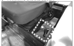
Pull the parking brake lever upward to apply the parking brake.
