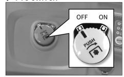
This switch is used to turn PTO shaft rotating on or off.
