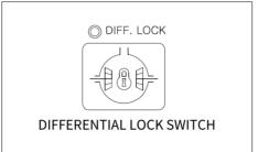
In case of wheel slippage, use the difflock with this switch
