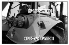
Operator can easily raise or lower 3P position from outside of the tractor for convenience using external 3P up/down switches installed on both of the right and left side of the sub fenders.
