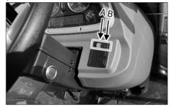
Press the hazard flasher switch in emergency to warn other vehicles in order to prevent an accident.
