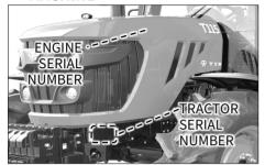
The engine and tractor serial number are stamped as shown in the drawing above.
