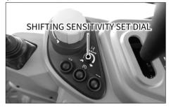
Moving speed of forward or reverse direction at starting can be adjusted using this dial.
