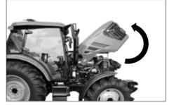
Lift the hood with hands slightly while pushing the lever inside.
