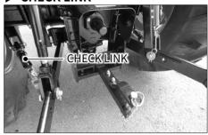
Check link is used to stabilize lower link.
