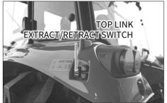
Top link position can be adjusted outside with an external switch installed on the left side of the sub fender.
