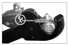
Confirm that a lock pin is installed after an implement is attached.
