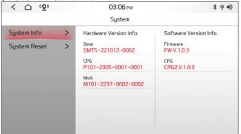
You can reset the touch monitor or check the hardware and software version of touch monitor.
