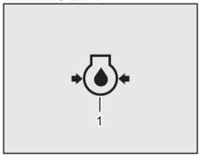
(1) Engine Oil Pressure Warning Lamp
