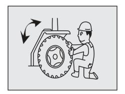
Adjust the wheel tread depending on the type and condition of the work. Also, increase the wheel tread when working on a slope or towing.
