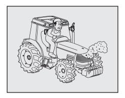
Put tractor rain cover on only after tractor has cooled down;
