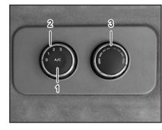
(1) Cooling Function (2) Air Flow Rate (3) Temperature
