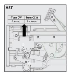
(1) Neutral Adjust Shaft (B) Fix Bolt
