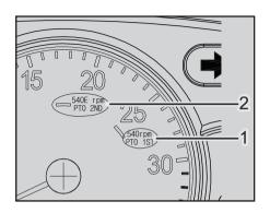
(1) PTO Position(1st stage) (2) PTO Position(2nd stage)
