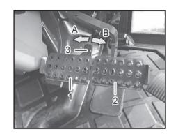
(1) Left Brake Pedal (2) Right Brake Pedal (3) Link Bracket
