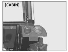
(1) Brake Lamp It is turned on when the Brake pedal is depressed.
