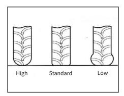
Adjust air pressure in front and rear tires to standard pressure.
