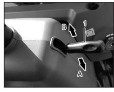
(1) Steering Column Tilt Lever (A) Release (B) Lock
