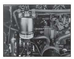
Drain the air from the fuel tank, fuel filter, and fuel filter element when the engine stops as the fuel runs out or during maintenance
