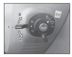
(1) Turn Signal Lamp Switch (A) LH (B) RH
