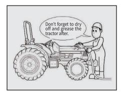
After work, clean the tractor and dry the moisture and supply grease into each grease nipple.
