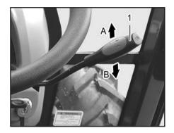
(1) Hand Throttle Lever ←: Slower Engine RPM (A)
