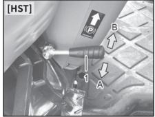
(1) Parking Brake Lever (A) Release (B) Lock
