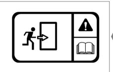
If exit from the cab side doors is blocked (following an accident or vehicle overturn) the alternative safety exits are indicated by decals.
