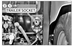
The socket is ready to operate the electrical systems of implements, trailer lighting, warning lamps and etc.
