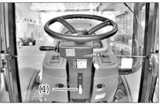
The angle of the steering wheel can be adjusted to suit the driver. The tilt lever is installed under the steering wheel. Use this lever (1) to adjust the position. To fix the position, push down the lever.
