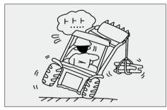
Do not lift anything only with one side of the tractor. If so, the tractor may fall on its side.
