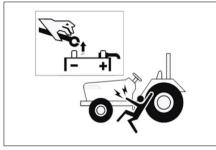
When working with your tractor electrical components, you must first disconnect the battery cables.
