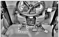
Depressing the clutch pedal disengages the clutch.
