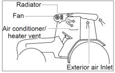
The fan speed can be adjusted in four steps for the air conditioner and heater.
