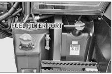
Use only low sulfur or ultra low sulfur diesel fuel.
