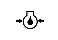
If the oil pressure lamp comes on check the oil level first of all.
