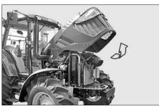
2. Lift the hood with hands slightly. Then, the hood is automatically opened by its damper.
