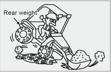
Keep the balance between the front and rear by installing a weight to the back of the tractor or attaching a weight or implement using the 3-point link.
