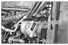
Check and adjust the tension of the A/C compressor belt regularly.
