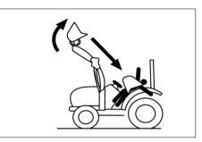
When attaching or detaching the loader, fix all parts which are connected to the bucket and boom.
