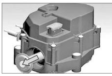
2. Remove the equalizing element.
