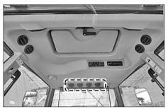
There are two circulation modes for the A/C and heater operation: fresh air mode and recirculation mode.
