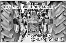
Turn the handle clockwise to extend the rod and turn it counterclockwise to retract the rod.
