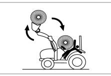
Never carry a big object with the loader unless a proper implement is attached.
