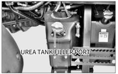
When the urea amount in the tank is below 25%, the urea level warning lamp comes on. In this case, add more urea into the tank.
