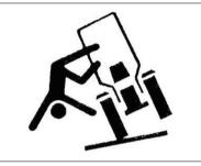
The Roll Over Protective Structure(ROPS) has been certified to industry and / or government standard. Any damage or alternation to the ROPS, mounting hardware or seat belt voids the certification and will reduce or eliminate protection for the operator in the event of a roll-over.
