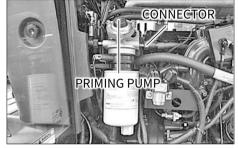
(2) How to bleed fuel systemIt is necessary to bleed the systemunder the following conditions:The engine is stopped due to the
