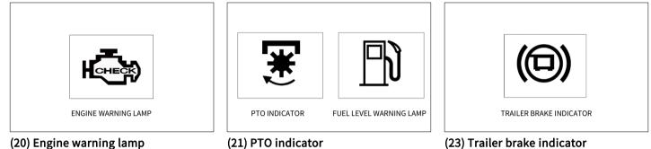
It comes on when the engine is malfunctioning.
