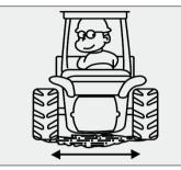
Keep the clearance between the rear wheels as large as possible for safety of the tractor.
