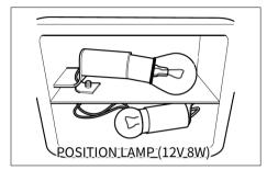
Remove the bulb by pressing it and turning it counterclockwise.
