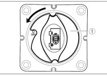
The function of the battery disconnect switch is to disconnect the power supply to the electrical system by interrupting the connection to the battery.
