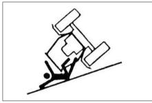
Do not drive where the tractor could slip or tip.
