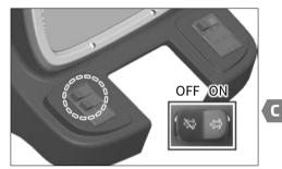
When the Forced DeSOx switch is 1 set in the neutral position, the **DeSOx operation is automatically** performed for every 200 hours.
