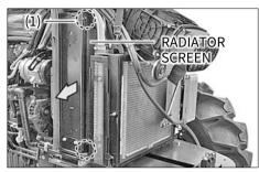
When working in a grassy field or working at night, the radiator or condenser grille may be clogged by grass, straws or bugs, reducing cooling performance.
