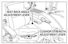
• SEAT BACK ANGLE ADJUSTMENT The seat can be fold down or up using seat back angle adjustment lever.
