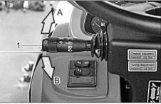
(2) Turn signal lamp operation The turn signal lamps can be operated with the main switch in the "ON" position regardless of the position of the column lever.
