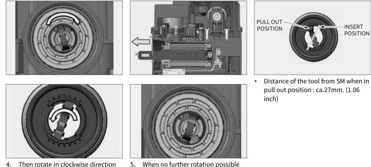
4. Then rotate in clockwise direction as shown in front view.
