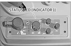
When there is an electric or electronic fault, the indicator (1) blinks according to the setting in the system to inform the type of the fault.
