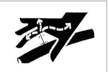
Escaping fluid under high pressure can penetrate the skin causing serious injury. Keep hands and body away from pin holes and nozzle which eject fluids under high pressure.
