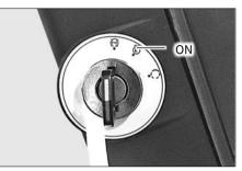
When key switch is in <code>「ON」</code> position, engine is automatically preheated as necessary.
