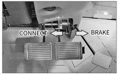
When two brake pedals are installed.
