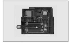
3. Insert the tool till it clips on guide.
