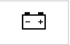
If the alternator warning lamp comes on check all connections and ensure that the fan belt is not broken. If all connections and the fan belt are intact consult your dealer to determine the cause of the problem.
