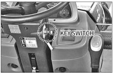
It is used to start and stop the engine.
