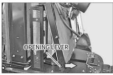
Turn the opening lever to access to the condenser and oil cooler. Clean them with clean water. Remove the grill by unscrewing the pin (1) and moving it in the arrow direction.  CHECKING AND CHANGING ENGINE OIL
