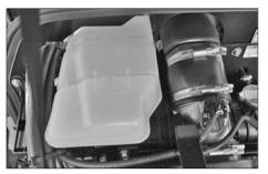
(1) Inspection Open the Coolant cap and check if coolant is filled up to the filler neck. If not, add more coolant to the radiator.
