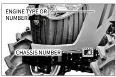
The chassis number is stamped as shown in the drawing above.
