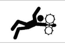
Do not wear a necktie, scarf or loose clothing when you work near moving parts.
