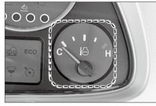
If the needle of the coolant gauge points at "H," stop the engine and check the followings:
