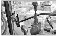
Press the button on the lever to open the door from outside. Push the lever down to open the door from inside.
