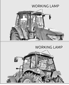
There are 4 work lamps installed on the front and back of the cabin roof. They can be operated by the buttons on the panel on the right side in the cabin.
