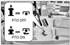
This is the PTO ON/OFF switch. To use the independent PTO, pull up the knob.
