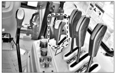
Like the throttle pedal, it is used to control the engine speed. This lever is operated with a hand and can be used to fix the engine speed to a certain level.
