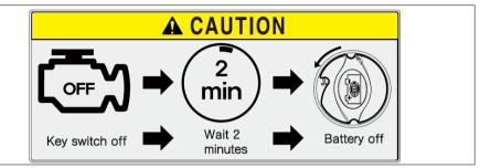
Turn the knob to "OFF" to disconnect the battery and back to "ON" to resume normal operation.
