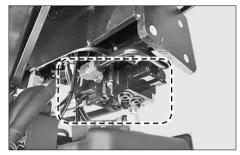
The loader valve is installed under the step on the right side and the joystick lever is installed on the right from the driver's seat in the cabin for easy installation and operation of a loader.
