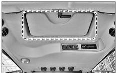
Use it to ventilate the cabin. To open the sunroof, turn the lever clockwise and push it up. To close the sunroof, hold the lever, pull it down and turn it counterclockwise.
