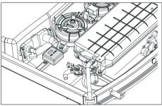
This supplies power to the cabin control panel and cabin electric devices. If any cabin electric device is not operating properly, check this part. If defect is found, replace it with a new one.
