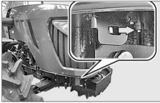
1. Push the hood opening handle under the hood front grill to the left as shown in the figure to unlock the hood.
