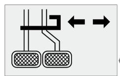
There is an engaging hook for connecting the left and right brake pedals.
