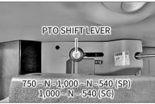
This lever is used to select the PTO speed. its operation is coupled with the PTO
