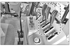
When using an attachment for an implement (rotavator, hydraulic plow, etc.), connect its hose to the proper port among the port A, B and C according to its use.
