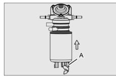
(3) Tighten the drain valve
