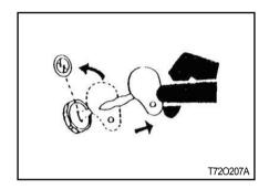
Before working on the tractor; Lower all equipment to the ground. Stop the engine and remove the key.
