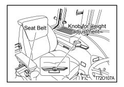
The seat cushion can be adjusted According to the weight of the driver.
