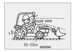
When transporting things with a loader, lower the loader and keep the driving speed slow. Keep the loader 30 to 50 cm off the ground and the driving speed below 5 km/ h. When going onto a slope or unpaved area, lower the speed and drive with care.
