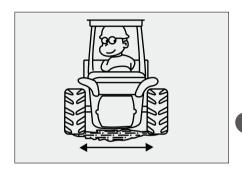
Keep the clearance between the rear wheels as large as possible for safety of the tractor.
