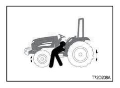
Do not allow riders on the tractor. Riders on tractor are subject to injury such as being stuck by foreign objects and being thrown off of the tractor.
