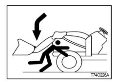
Do not stand under the lifted loader or get close to it. Also, lower the loader arm onto the ground before leaving the tractor. Otherwise, it may lead to a fatal injury or even death.
