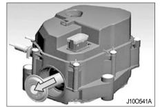
2 Remove the equalizing element
