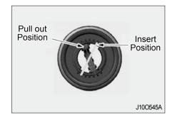
Distance of the tool from SM when in pull out position: ca.27mm. (1.06 inch)
