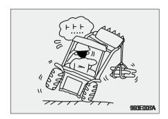
Do not lift anything only with one side of the tractor. If so, the tractor may fall on its side. Make sure to distribute the load evenly.
