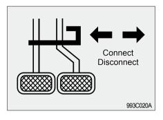
There is an engaging hook for connecting the left and right brake pedals.
