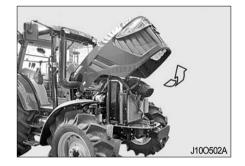
② Lift the hood with hands slightly. Then, the hood is automatically opened by its damper.
