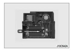
3 Insert the tool till it clips on guide.
