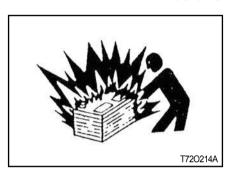
Keep sparks, lighted matches, and open flame away from the top of battery. Battery gas can explode.
