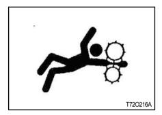
Do not wear a necktie, scarf or loose clothing when you work near moving parts. If these items were to get caught, severe injury could result.
