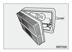
3 Install the lamp lens by pressing it against the cover from one side.
