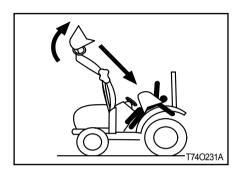
When attaching or detaching the loader, fix all parts which are connected to the bucket and boom. The bucket or boom can be accidentally dropped down, leading to an injury or even death.
