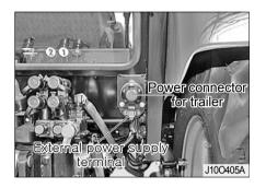
When driving the tractor attached with a trailer, make sure to connect the power connector to the trailer for proper operation of lamps on the trailer.
