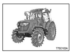
If the tractor has rolled over or the ROPS has damaged (such as striking an overhead object during transport), It must be replaced to provide the original protection. After an accident, check for damages to the 1.ROPS, 2.Seat, 3.seat belt & seat mountings. Before you operate a tractor, replace all damaged parts.
