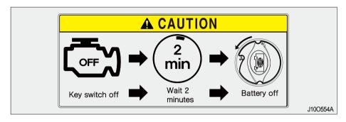
Turn the knob to "OFF" to disconnect the battery and back to "ON" to resume normal operation. The battery disconnect knob (1) is located on the bracket to the right of the battery. The battery disconnect knob may be removed for safety purposes in the manner described below.
