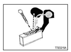
Sulfuric acid in battery electrolyte is poisonous. It is strong enough to burn skin, cause holes in clothing and cause blindness if found entry into eyes.
