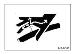
Escaping fluid under pressure can penetrate the skin causing serious injury. Keep hands and body away from pinholes and nozzles, which eject fluids under high pressure. If any fluid is injected into the skin. Consult your doctor immediately.
