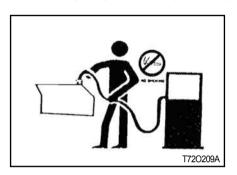
Handle fuel with care; it is highly flammable. Do not refuel the tractor while smoking or near open flame or sparks.
