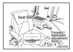
Before operating a tractor it is important to adjust the seat to the most comfortable position & check whether it is properly locked in its position.
