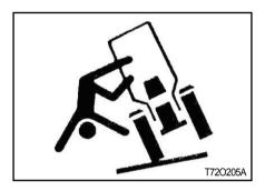
The Roll Over Protective Structure (ROPS) has been certified to industry and/or government standards. Any damage or alternation to the ROPS, mounting hard-ware, or seat belt voids the certification and will reduce or eliminate protection for the operator in the event of a roll-over. The ROPS, mounting hardware, and seat belt should be checked after the first 100 hours of tractor and every 500 hours there-
