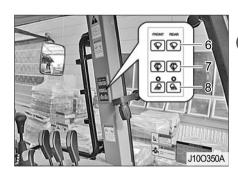
The switches for the windshield/rear wipers/washers and work lamps are located on the right side from the driver's seat.
