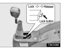
(2) Joystick lever safety device There is a button to lock the operation of the joystick lever. Pulling it forwards unlocks the lever while pushing it backwards locks the lever.
