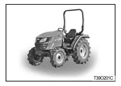
If the tractor has rolled over or the ROPS has damaged (such as striking an overhead object during transport), It must be replaced to provide the original protection. After an accident, check for damages to the 1.ROPS. 2.Seat. 3.seat belt & seat mountings. Before you operate a tractor, replace all damaged parts.
