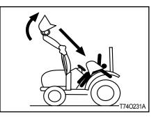
When attaching or detaching the loader, fix all parts which are connected to the bucket and boom. The bucket or boom can be accidentally dropped down, leading to an injury or even death.
