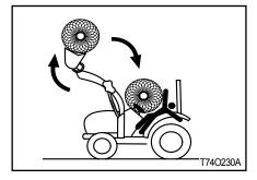
Never carry a big object with the loader unless a proper implement is attached. Keep a carried object low during driving. Otherwise, it may lead to an injury or even death.
