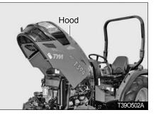
② Lift the hood with hands. Then, the hood is automatically opened and fixed by its damper.
