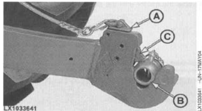
Coupler hook operated by means of a control cable
